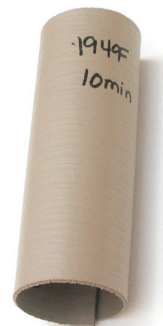
Fig. 1 Extreme warping in an ASA capped vinyl siding sample, sample was exposed at 90^{\circ}\text{C} ( 194^{\circ}\text{F} ) for 10 min
